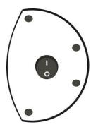
d.Before fixed the heater,make sure the rocker power switch on the right side and then fixed the bracket and heater by two M6\*14 screws and butterfly nuts
