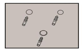
c. Fixed the bracket by three ST4\*35 screws and make sure the installation points fixed securely
