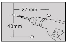
b.Insert the three plastic wall anchors to the three holes
